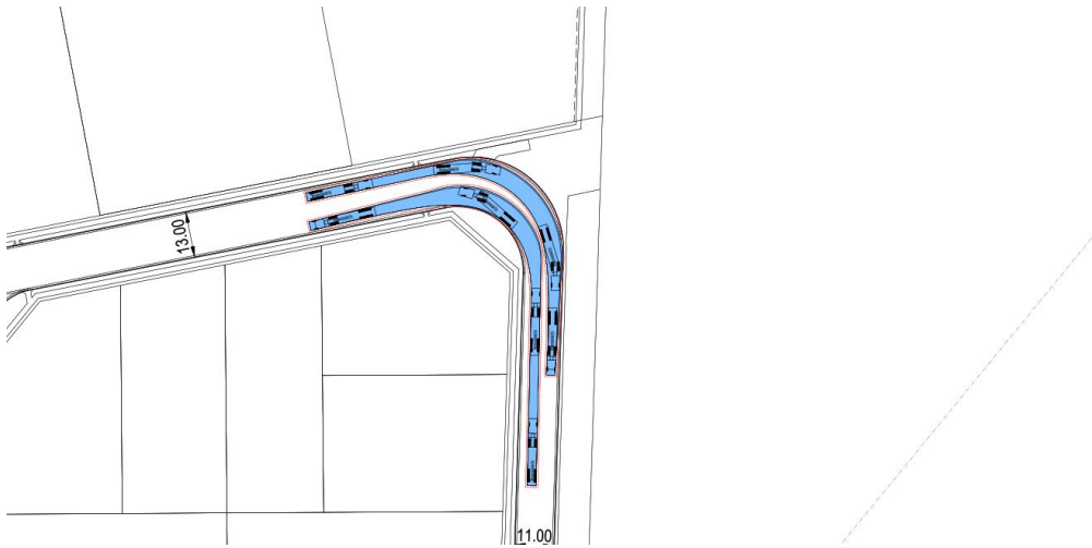
Figure 2 Section of Road MC01 - Swept Path Diagrams
